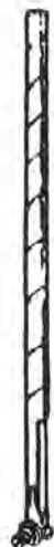
10-1028-2-000 (10-1028) Needle bar comp. 01-2193-0-000 (01-2193) Needle screw 01-5167-0-000 (01-5167) N. bar ten. spring 10-1029-0-000 (10-1029) N. bar. ten. disc 10-1030-0-017 (10-1030) Ten. holding screw 10-1032-0-000 (10-1032) Needle bar nut
