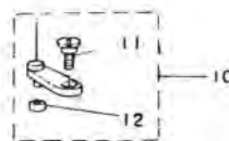
10 B1230-372-0/ Loop positioning finger asm 11 SD-0640241-S Hinge screw D=6.35 H=2.4 12 B1232-372-000 Lever roll
